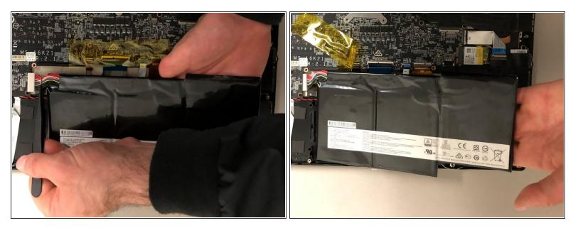
(i) The battery is attached to the laptop with a strong adhesive.
