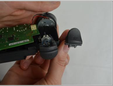
Insert the plastic opening tool into the space created when the button is pressed down. Make sure
