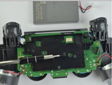
Remove the 6.43mm screw connecting the motherboard to the inner workings of the controller, using a Phillips-Head screwdriver.
