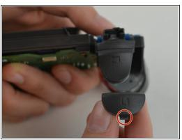
Pry the button from the controller using the plastic opening tool. Slide the tool between the buttons.
