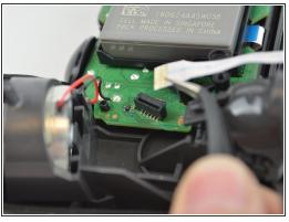
Pull the ribbon cable out of the motherboard port to fully separate the two halves, using a pair of tweezers.
