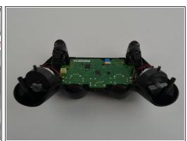
• Unhook the battery case from the motherboard, and pull it off.
