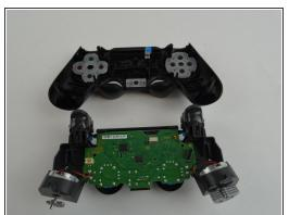
• Pull out the second CPU ribbon to separate the inner workings from the top of the outer shell.
