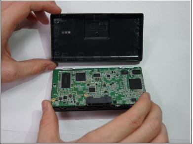
Apply pressure to the iFixit opening tool, pushing down until the the plastic casing pops off.
