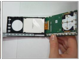
Remove the buttons from the casing.
