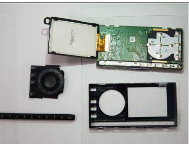
Remove the motherboard, and the casing should be free.
