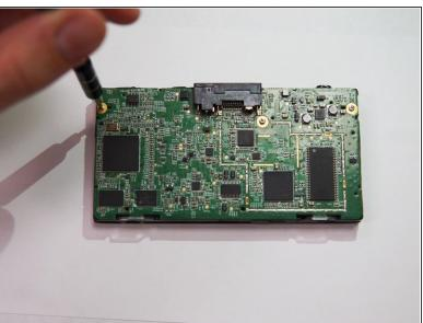
Use the Phillips PH00 screwdriver to remove the three marked screws.
