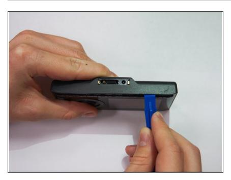
Take the iFixit opening tool and place it between the back casing and the device as shown.
