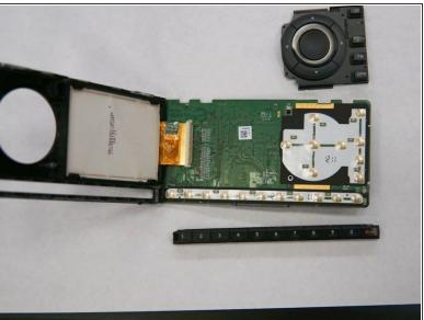
The buttons are resting in the corresponding sections of the motherboard, so pull them off.
