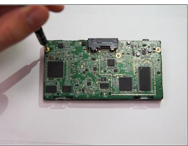
• The buttons are on the opposite side of the motherboard. To remove the motherboard, use a 0.8~0.9 mm Phillips #00 screwdriver to remove the three screws that attach the motherboard to the front part of the plastic casing.
