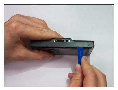
Take the iFixit opening tool and place it between the crevice as shown.
