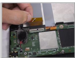
To remove the ribbon cable, move the black retainer upwards. Then pull the ribbon cable rearwards to remove it.
