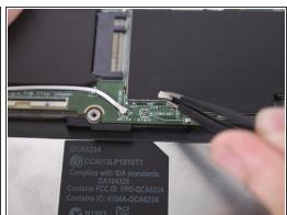
Use the tweezers again to grab hold of the black <u>coaxial connector</u> and pull upwards to disconnect.
