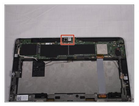
Now turn your attention to the two ZIF connectors at the top. The left ribbon cable connects to the webcam, the right ribbon cable connects to the back camera.
