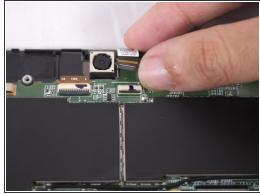
To remove the right ribbon cable, use the pointy end of your spudger to flip the black <u>ZIF</u> lock upwards. Then pull the ribbon cable rearwards to disconnect it.
