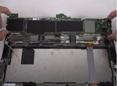
Finally the motherboard can be lifted out by hand.
