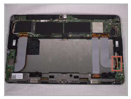
You must then remove the ribbon cable connected to the USB port located here.
