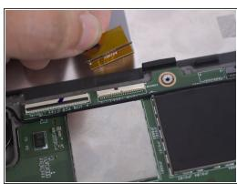
• Use the pointy end of your spudger to lift up the <u>ZIF</u> lock. Afterwards, pull the ribbon cable rearwards to disconnect it.
