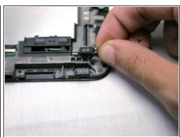
Locate the vibration motor at the bottom right corner of the screen shell. Grab the motor by the cable and pull upwards to remove.
