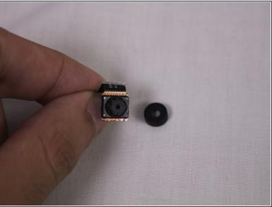
(i) Take caution when removing the front camera with the rubber cover. The cover can easily fall off from any slight movement.
