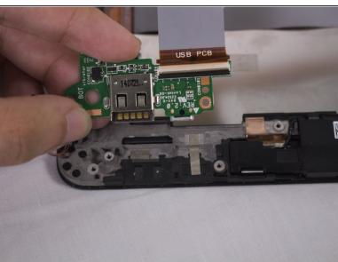
After disconnecting all the pieces, remove the USB port circuit board with your fingers
