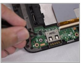
Using a pair of tweezers disconnect the connector from the circuit board
