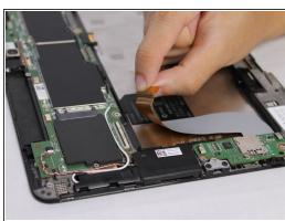
Wedge the tip of the plastic spudger in between the ZIF connector lock and flip up the lock. Pull the ribbon cable out.
