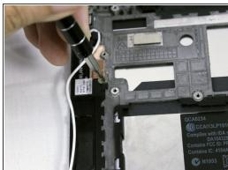
The final step is to remove the 2.5 mm bronze screw using a Philips #000 screwdriver.
