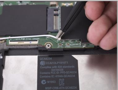
Now remove the white coaxial connector using the tweezers to pull the connector upwards.
