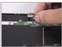
• To remove the left ribbon cable, use the pointy end of your spudger to flip the black <u>ZIF</u> retainer into the up position. Then simply pull it rearwards to remove it.
