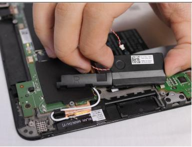
Once the cable has been detached, use your fingers to lift the right speaker upwards to remove it.
