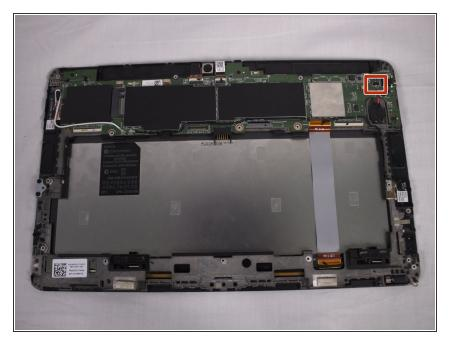
Now you must disconnect the small battery wire located here on the device.
