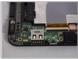
Using a Philips #000 screwdriver remove the two 2.5 mm screws indicated.
