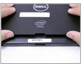
Turn your device over to the backside. On the notch at the bottom portion of the tablet, use your fingers to lift up the back cover.
