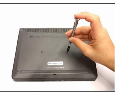
Use the #J0 screwdriver to unscrew the seven 4mm screws located around the back panel.
