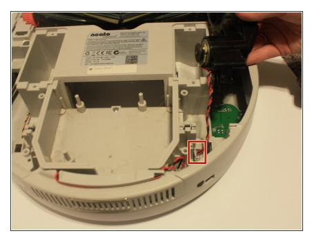
Pinch and pull the white connector, indicated in the image, to disconnect the wheel from the robot. Repeat for both wheels
