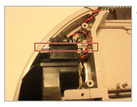
Slide out dowel rod connecting the wheel to the robot.
