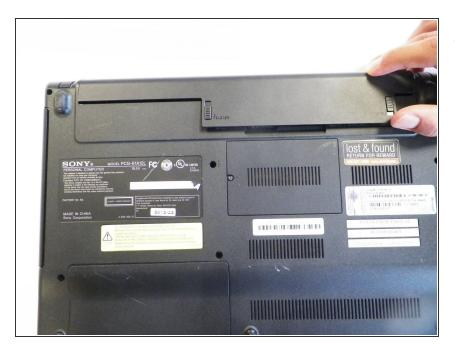
Unlock the battery by sliding the lock upwards.
