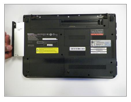
Grab and slide out the optical drive to remove.
