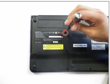
Using the Phillips #1 screwdriver, unscrew the 6.5 mm screw.
