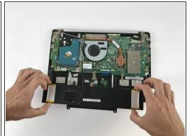
Gently take the battery out of the laptop, making sure that all wires connecting to it are disconnected.
