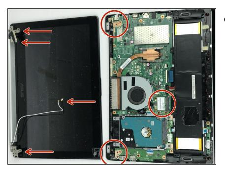
Remove the screws connecting the display to the laptop. Furthermore, detach the wires connecting the screen to the motherboard.
