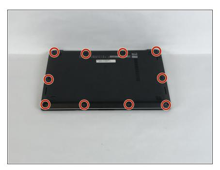
Unscrew the (10) screws on the bottom of the computer chassis using the JIS #0 screwdriver.
