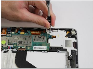
• Remove the two 3mm screws securing the white speaker with the Phillips #00 screwdriver.
