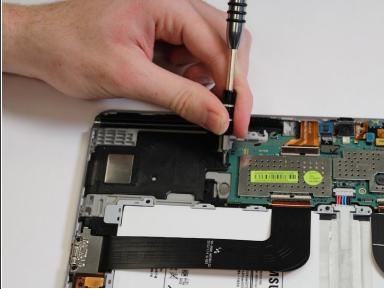
• Remove the one 3mm Phillips #00 screw securing the black speaker.
