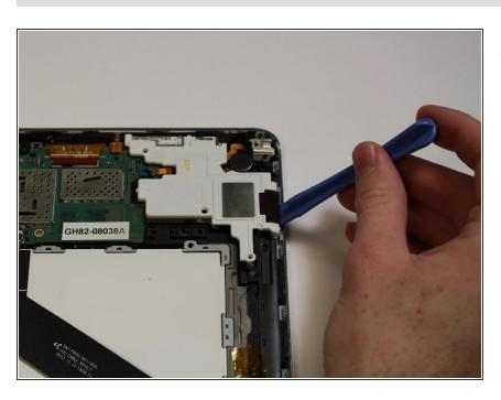
Using the blue opening tool pop the white speaker up and away from the device.
