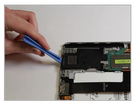
Using the plastic opening tool, pop the black speaker up and away from the device.
