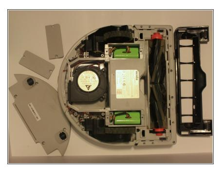
The Neato's core components are now exposed and ready to be cleaned and/or replaced.
