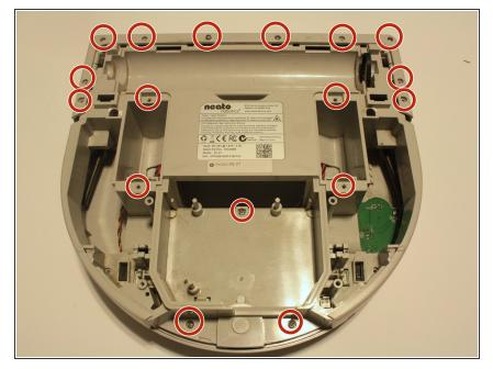
Remove the 17 visible screws and the 2 covered/hidden screws near the battery compartments that connect the bottom to the top of the Neato robot.
