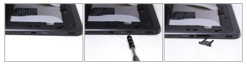
• Use your pin punch driver to push into the hole on the sim card, then pull out the sim tray.
