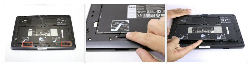
Below the battery pack, there are two lock mechanisms. Push EACH lock to the LEFT until it makes a click noise. Lift the battery from the bottom up and remove.
