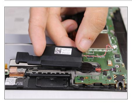
Lift the right speaker upwards using your fingers to remove it.
