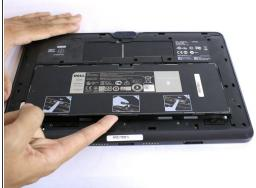
Below the battery pack, there are two lock mechanisms. Push EACH lock to the LEFT until it makes a click noise. Lift the battery from the bottom up and remove.
