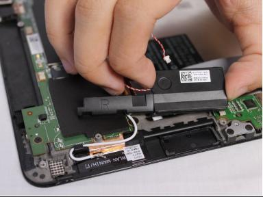
• Once the cable has been detached, use your fingers to lift the right speaker upwards to remove it.
