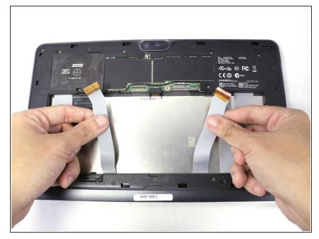
There are adhesive strips between the device and the two ribbon cables we disconnected. Pull each cable away from the device just enough to break the adhesive bonds.
