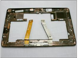
Insert your plastic opening tool between the screen and frame, and run the tool around the edges to separate the frame from the tablet.
