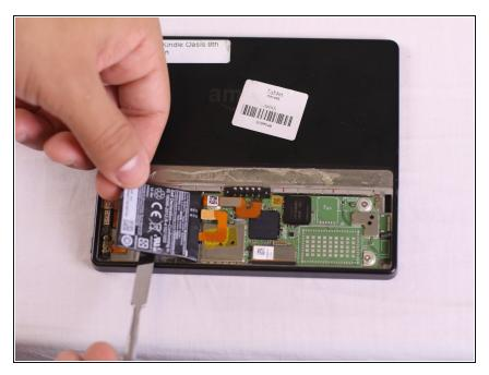
Lift the battery up using a spudger and use your fingers to slowly pull the battery off the adhesive.
