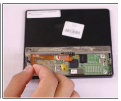
• Using the metal spudger, tweezers, and your finger tips, gently lift the orange power bridge connector off of the motherboard first and then off of the kindle.
