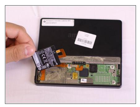
Once free of the adhesive and connectors, remove the old battery from the device.
