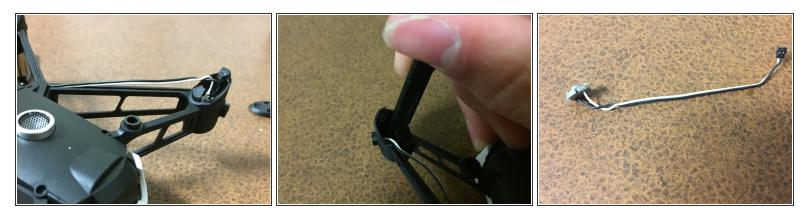
• Use the spudger to remove the base of the motor by pushing it through the top.
