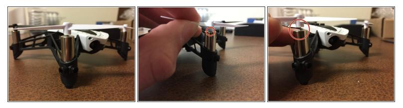
This motor is the defective one. The motor shaft is allowed to move freely up and down. Mine was the front right motor.
