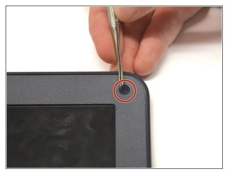
Using a flat blade, remove the two screw covers on the front of the bezel. They are attached by adhesive, so you may have to dig at it a little bit.
