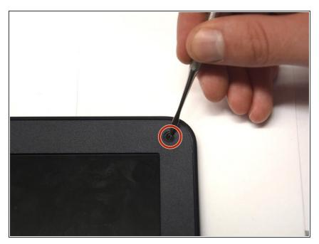
• Unscrew and remove the two Phillips #1 4.5 mm screws that are now visible.
