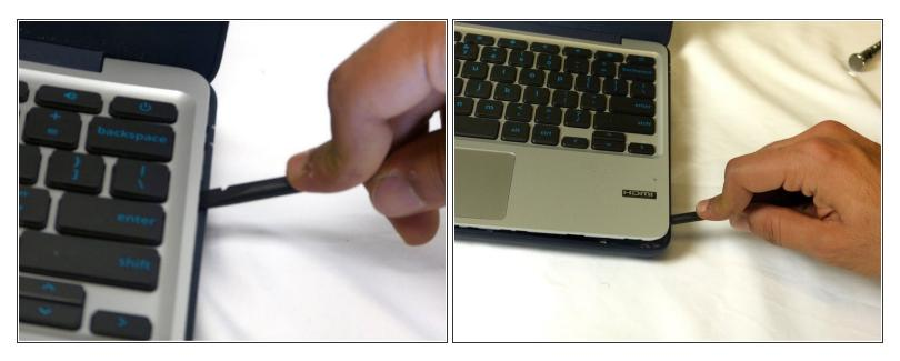
• Carefully use the plastic opening tool to pry the palm rest apart from the bottom cover. Start from one spot and systematically work your way around until the whole palm rest is detached.
