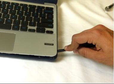
Carefully use the plastic opening tool to pry the palm rest apart from the bottom cover. Start from one spot and systematically work your way around until the whole palm rest is detached.
