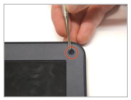
Using a flat blade, remove the two screw covers on the front of the bezel. They are attached by adhesive, so you may have to dig at it a little bit.
