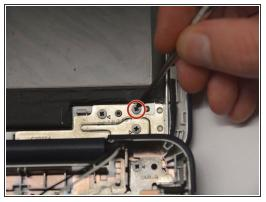
• Unscrew and remove the four screws holding the screen in place.
