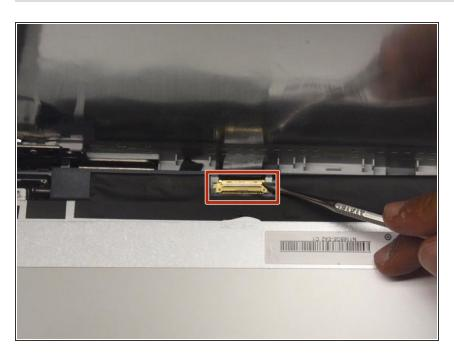
Fold down screen and remove the screen connector band. You may have to use a small flat blade or a spudger, since the latch is very small.
