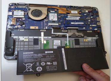
• Lift the battery up at an angle to disconnect the battery from the motherboard, then pull it away from the laptop.
