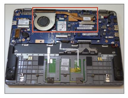
Locate the cooling fan and the heat sink on the top center of the Chromebook.
