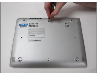
• Remove the eight 7mm screws using the J0 Screwdriver.
