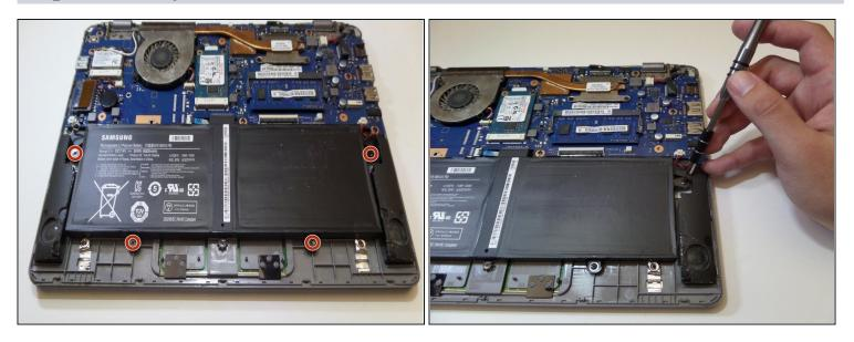
• Remove the four 3mm screws holding the battery with the J0 screwdriver.
