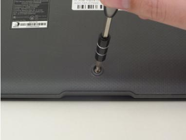
• Unscrew the five 5-mm screws using the PH0 screwdriver.
