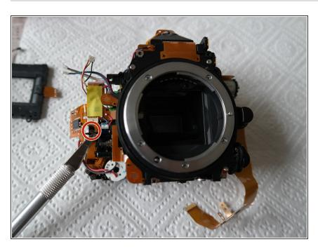
Pull off the flex cable and remove the 3rd screw underneath.
