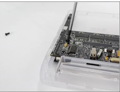
Unscrew the two 2.94mm Phillips #00 screws that hold the motherboard in place.
