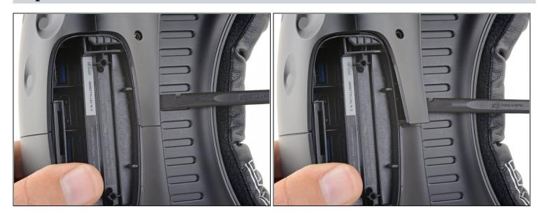
• Use the flat end of a spudger to pry up the top edge of the right half of the outer shell, behind the component cover and near the seam in the center, until it is unclipped from the headset.
