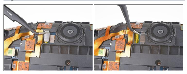
• Use tweezers or a spudger to pry up the camera cable cover and remove it.
