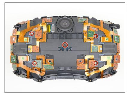
Use a PH000 driver to remove the five 3.9 mm screws securing the sensor array.
