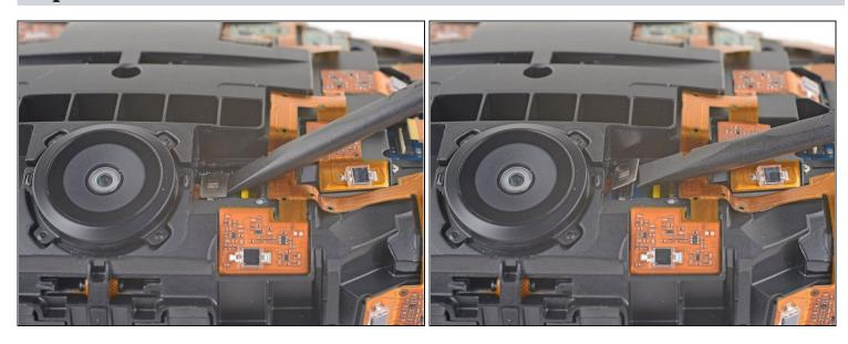
• Use the flat end of a spudger to pry the camera cable connector straight up from its socket on the motherboard.
