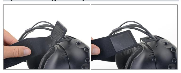
• Slide the top part of the head strap through its metal loop on the headset to remove it.
