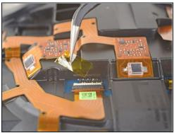
• Use <u>tweezers</u> to remove the clear tape over all four of the sensor array cable connectors.
