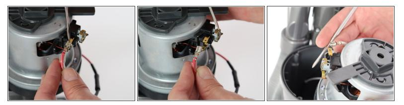
• Use a **plastic** spudger or opening tool to press on the small circle and wiggle clips free.
