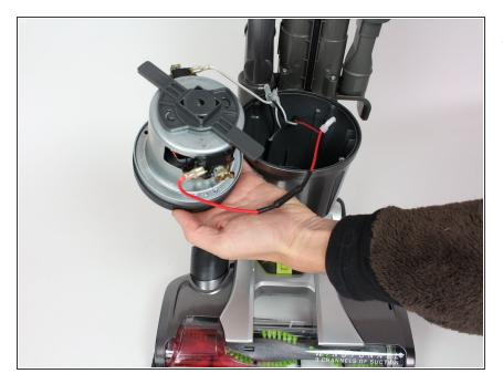
• Pull the motor housing vertically to dislodge the motor.
