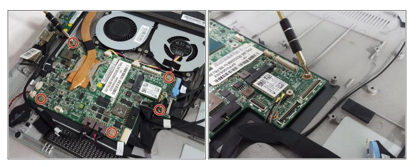
With the Phillips #1 head, remove the M2-6mm screws seating the motherboard into the case.
