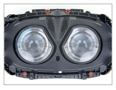
Use a PH000 driver to remove the four 3.9 mm screws securing the facerest midframe.
