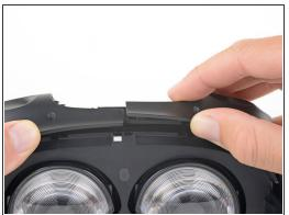
Grasp the top edge of the right half of the outer shell, behind the component cover and near the seam in the center. Pull it to the right and upward, away from the headset to release the clip securing that part of the shell.
