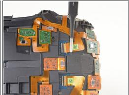
Repeat the previous step for the remaining three sensor array cables to disconnect the remaining cables.
