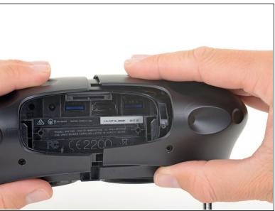
Grasp the right half the outer shell and pull it to the right and toward the front of the headset in a twisting motion until you feel the clips on the front of the cover release.
