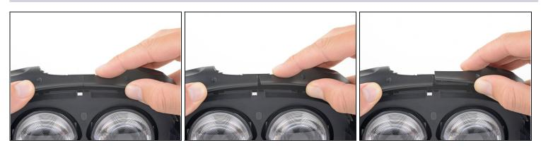
• Grasp the top edge of the right half of the outer shell, behind the component cover and near the seam in the center. Pull it to the right and upward, away from the headset to release the clip securing that part of the shell.
