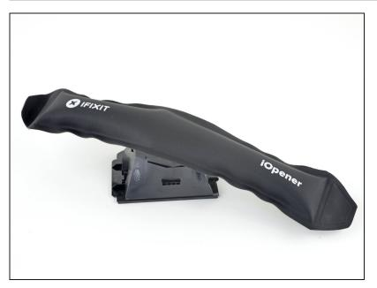
Apply an <u>iOpener</u> to the lens to soften the adhesive securing it to the frame.
