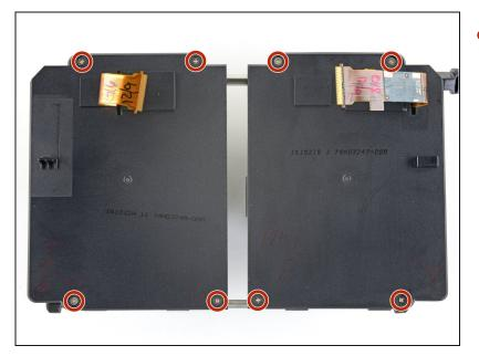
• Use a PH000 driver to remove the eight 2.4 mm screws securing the OLED covers.
