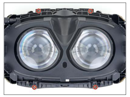
Use a PH000 driver to remove the four 3.9 mm screws securing the sensor array.
