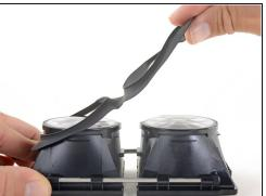
• Gently lift the eyepiece gasket off of the lens and OLED frames to remove it.
