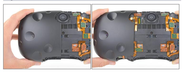
• Repeat the last three steps for the left side of the outer shell and remove it.
