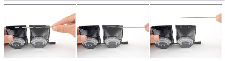
Slide the support rod out of its brackets on the lens and OLED frames.
