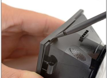
• Use the flat end of a spudger push up one edge of the OLED cover and start unclipping that edge.
