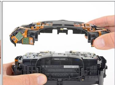
• Lift the sensor array away from the headset to remove it.
