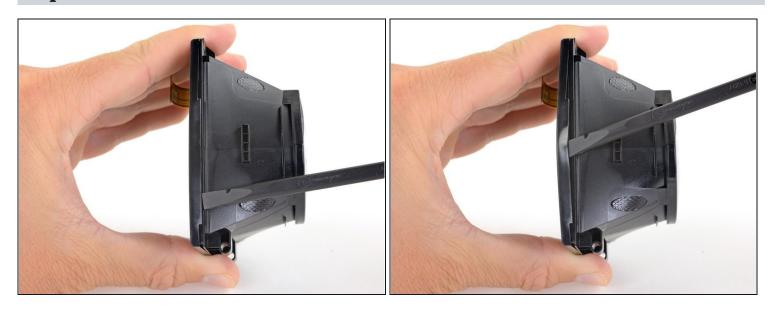
• Slide the spudger under the clip along that edge to free the rest of the edge.
