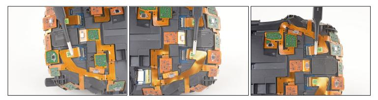
• Repeat the previous step for the remaining three sensor array cables to disconnect the remaining cables.
