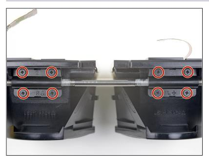
Use a PH000 driver to remove the eight 3.1 mm screws securing the focus rod brackets.
