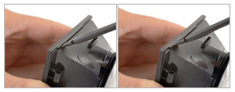
• Use the flat end of a spudger push up one edge of the OLED cover and start unclipping that edge.
