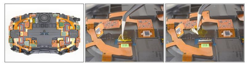
• Use tweezers to remove the clear tape over all four of the sensor array cable connectors.
