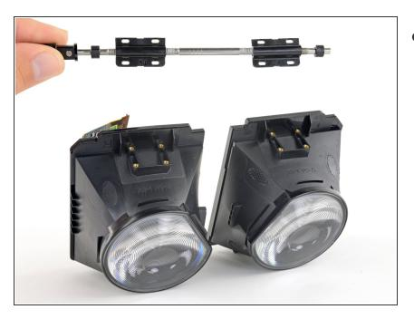
Remove the focus rod and its brackets.
