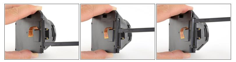
• Slide the spudger around the remaining edges of the OLED cover to unclip those edges.
