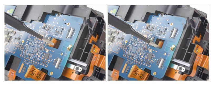
• Use a pair tweezers to slightly twist the interconnect cable and press it down until the tabs on either side of the cable clear the hole in the motherboard.
