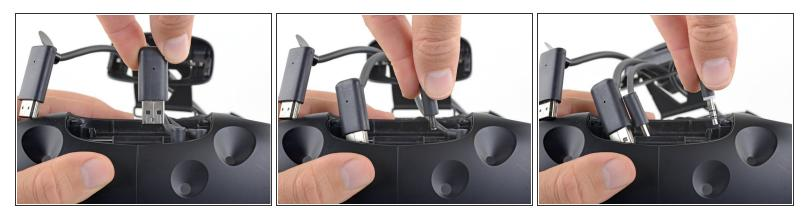
• Repeat the lifting and unplugging process with the remaining USB, power, and audio cables.
