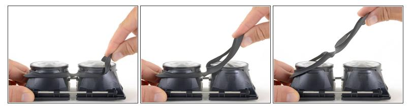
• Gently lift the eyepiece gasket off of the lens and OLED frames to remove it.
