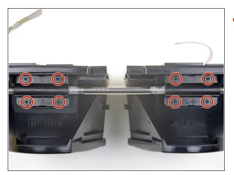
Use a PH000 driver to remove the eight 3.1 mm screws securing the focus rod brackets.
