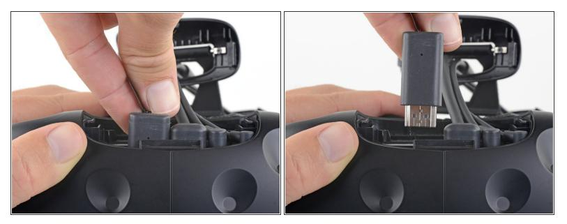
• Lift the HDMI cable straight up to unplug it from the headset.
