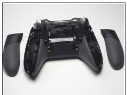
A Be careful not to break the plastic tabs, that hold each grip cover to the back of the controller.
