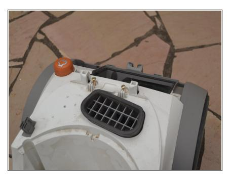
2 Torx screws under the hinge
