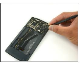
Using a black spudger, disconnect all connectors by lifting up gently.
