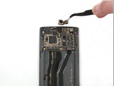
Using a pair of tweezers, gently lift the front facing camera out of the device.
