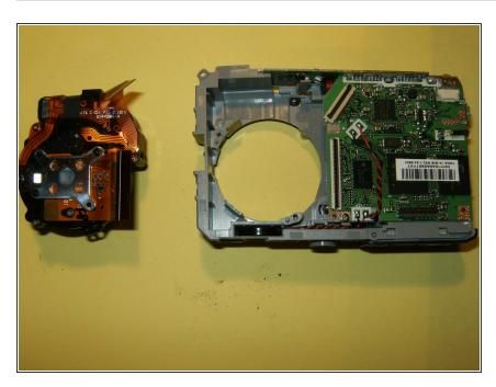
This is what your final result should look like. the lens is now free from the midframe and a new lens can be easily installed.
