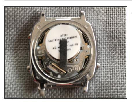
Gently lift up the sticker to access the battery. There is a small hole for prising the battery out, but as I did not need to remove the battery I only used it to jiggle the battery about. Therefore I did not see if there were additional fixings or note the battery number.
