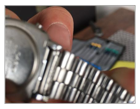
The trick is to hold the watch body and strap in one hand using your finger(s) to apply downward pressure to the strap while using your freehand to press down with the screwdriver head on the holding pin. If you get this right the pin and the top of the strap will come straight out
