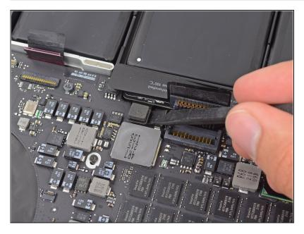
Use the flat end of a spudger to pry the trackpad ribbon cable connector up from its socket on the logic board.
