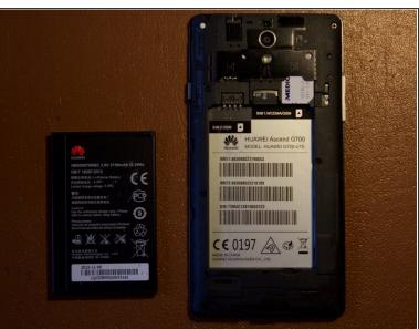
Now you can remove the battery, that has to be pryed off in the marked location.
