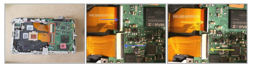
Release the flex clamps on the board. These clamps are very fragile so please be careful when flipping them up. Use of a spudger is a great help. Notice the two clamps are not in the same direction.
