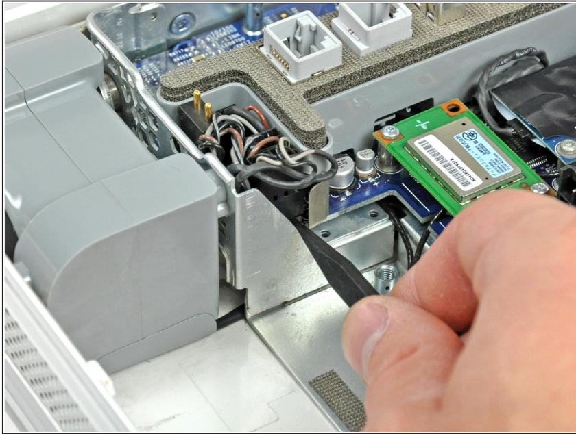
**⚠** The connectors removed in the next few steps slide onto long pins attached to the logic board. Be sure to only pull them straight up from the logic board to avoid bending the pins.
