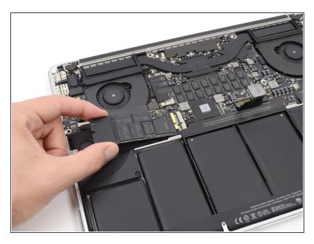
Slightly lift the leftmost side of the SSD and firmly slide it straight away out of its socket on the logic board.
