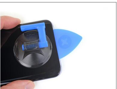
• Leave the pick in place and grab a second pick as you proceed to the next step. Leaving the pick inserted can help prevent the glue you just separated from re-adhering.
