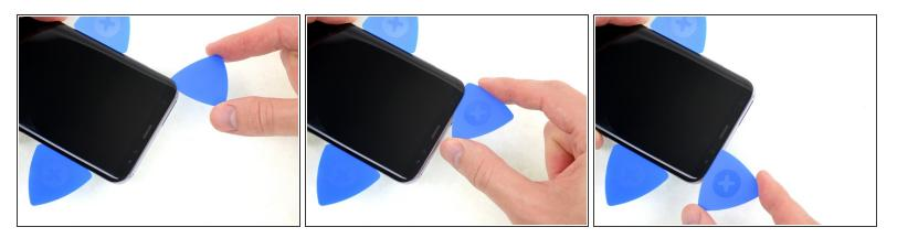
Gently work your opening pick under the top edge of the display to separate the adhesive underneath.
