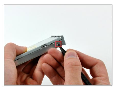
Use the pointed end of a spudger to depress and release the bezel retaining tab on the side of the optical drive.
