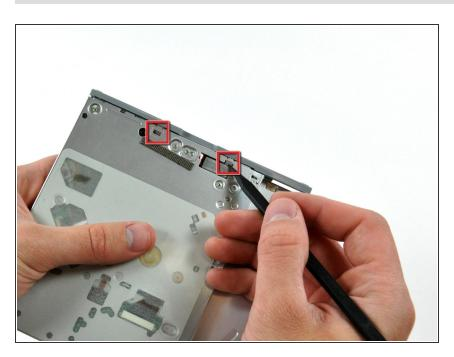
If necessary, use the pointed tip of a spudger to release the two plastic bezel tabs from their slots on the bottom of the optical drive.
