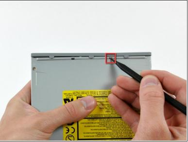
Use the tip of a spudger to push the two plastic bezel tabs away from their retaining slots on the top of the optical drive.
