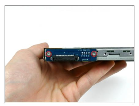
Remove the two 3.7 mm T6 Torx screws securing the optical drive connector board to the optical drive.
