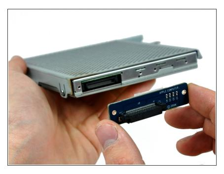
Remove the optical drive connector board.
