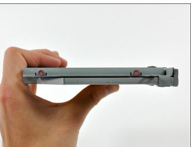
Remove the two 4.5 mm shouldered T6 Torx screws from each side of the optical drive (four screws total).
