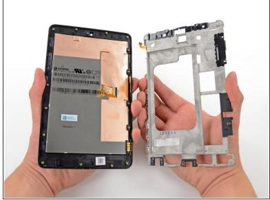
The frame comes off with the turn of a <u>screwdriver</u>, revealing another copper alloy shielding the LCD.
