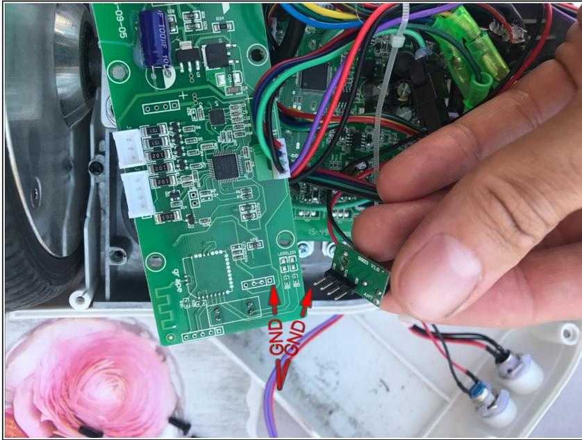
**⚠** Remember the sequence of wires to be soldered on the Bluetooth board.
