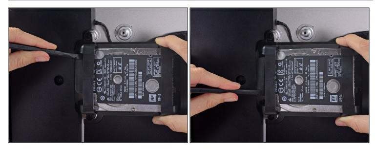
• Use a spudger to disconnect the single SATA power and data combo cable by gently prying its large plastic connector away from the hard drive.
