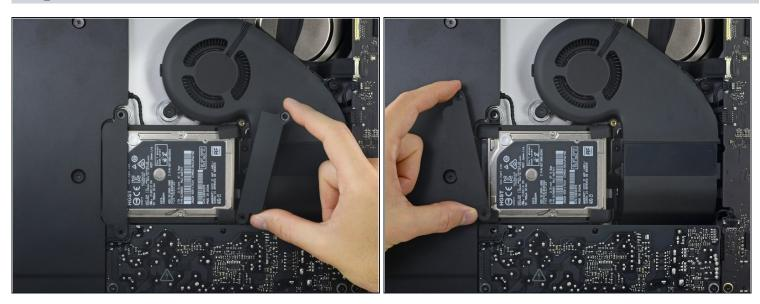
• Remove the left and right hard drive brackets from the iMac.
