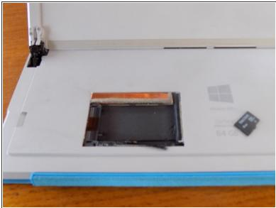
• The drive should just lift out, I used a Micro SD card to cover my serial number.
