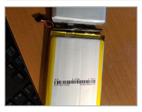
Two Lithium polymer batteries are connected back to back and in parallel to the regulator. The
