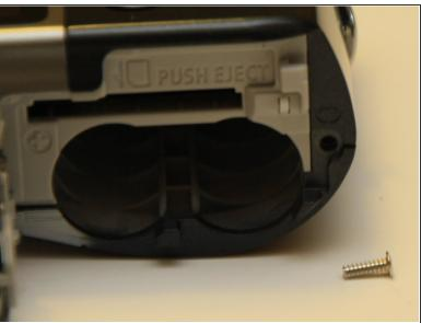
The last coarse thread screw is located under the battery/memory card cover. Remove this screw and we will be ready to open this baby up!
