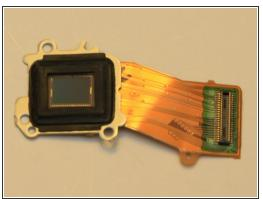
Remove the epoxy from the three coarse thread screws. Slowly loosen the three screws a little bit at a time. There are three springs underneath the metal plate that you might not want to launch. First time I did this I lost two of the three. The pink looking lens is a filter, if you turn the lens over it will fall out o be careful if you want to keep it.
