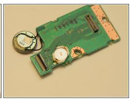
• Gently lift the keypad up from the bottom to remove it from the connector shown. You may need to pry up the speaker from it's holder, it is held in place with double-sided tape. Lift the keypad upside down and unhook the connector by lifting the gray cam and removing the flexible cable.
