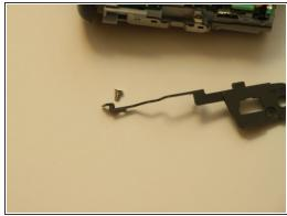
Remove the two fine thread screws on the top of the keypad. Then remove the one coarse thread screw holding the plastic piece in place on the side of the camera. Remove the plastic piece.
