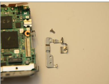
Remove the coarse thread screw from the upper keypad bracket.
