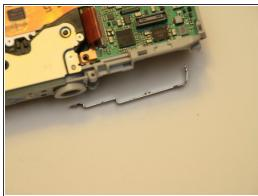
Remove the coarse thread screw from the lower keypad bracket.
