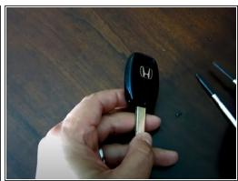
Use a Phillips #0 screwdriver to remove the screw at the base of the key fob.
