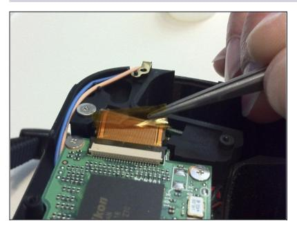
• Peel of the Foil securing the Flexcable.
