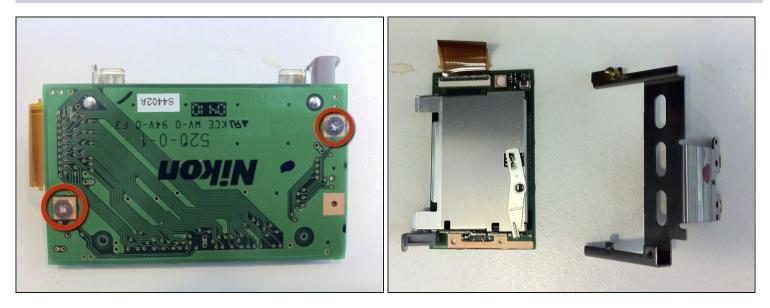
• Remove the two Phillips screws to separate the Holder from the Slot.
