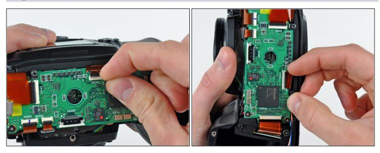
• Use your fingernail to flip up the ZIF locking flap on the LCD ribbon cable socket.
