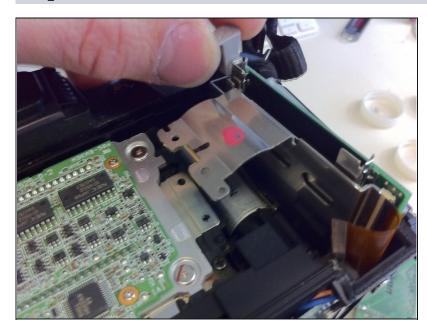
• Pull the Slot out of the body.
