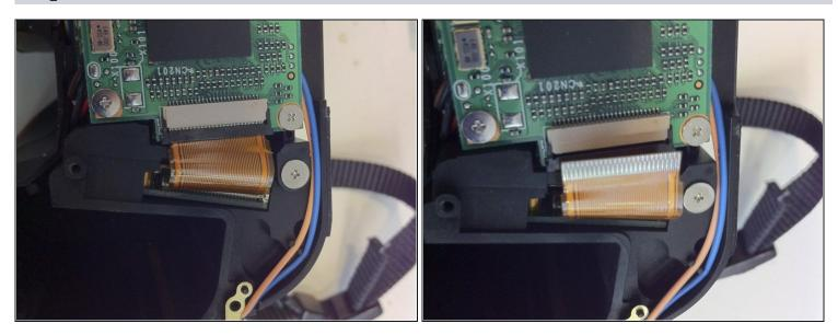
• Pull the ribbon cable out of its socket.
