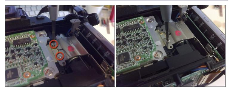
• Remove the two Phillips screws securing the holder of the CF Card Slot.
