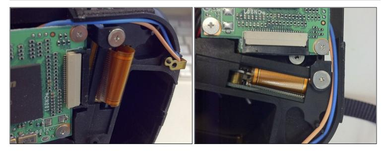
• Carefully fold the Pull the ribbon cable towards the CF Slot
