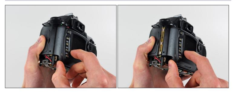
• Carefully pull the sides of the rear cover away from the body of the D70.
