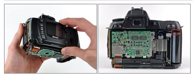
• Pull the rear cover off the body of the D70, minding the LCD board ribbon cable that may get caught.
