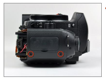
• Remove the two 4.8 mm Phillips screws securing the port side of the rear cover to the D70.
