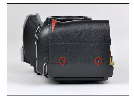
• Remove the two 4.8 mm Phillips screws securing the battery side of the rear cover to the D70.
