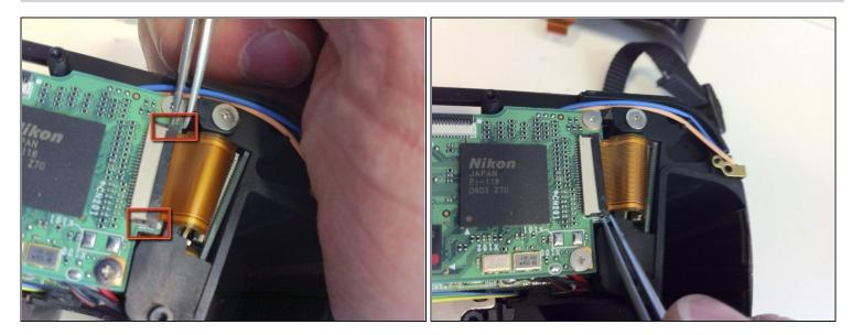
• Use <u>Tweezers</u> to open the locking on the ribbon cable socket.
